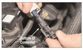
Plug the Interceptor harness connector into the factory 3-Pin sensor wiring harness connector. **NOTE: The correct orientation of the connector is shown above.**
