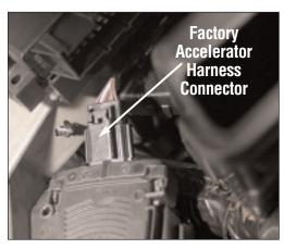
Disconnect the factory harness from the acceleratoe pedal sensor. Using a flashlight, you should see the accelerator pedal connector just behind the module which was unplugged in t he previous step. This picture is taken from the pedal area, looking up toward the windshield.
