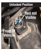
Disconnect the factory connector for the 4-Pin cam sensor. This connector has a locking clip that must be slid back to unlock. Notice the slight difference in the position when the tab is in the "UNLOCKED" position. Then, squeeze down the locking tab, and push the connector in slightly (toward sensor) and then remove.
