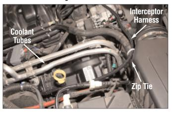
Route the Interceptor harness toward the air inlet box, and then back to the 4-Pin cam sensor. *Use the provided zip ties to route the Interceptor harness away from coolant tubes*.
