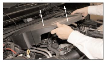
Lift off the engine cover and place it to the side while installing the Hypertech Interceptor.
