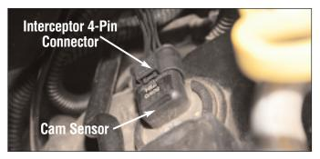
Plug the Interceptor 4-Pin connector into the vehicle cam sensor. Then plug the Interceptor harness 4-Pin connector into the factory wiring harness 4-Pin connector. Reinstall the engine cover *making* sure that the retention grommet(s) are attached to the cover correctly. These can stick to the standoffs when removing the cover, and must be reattached to properly reinstall the cover.
