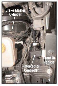
**Suggested mounting location:** Locate the flat panel next to the brake master cylinder on the passenger side near the firewall. Attach the Interceptor Controller to this panel with the supplied velcro and route the cable as shown.
