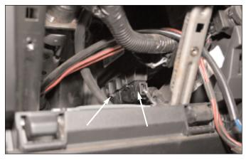
Using the 10mm socket and ratchet, remove the metal plate located behind the dash panel. Then, remove the two (2) connectors from the module behind the metal plate. Move these to the side for easier access and visibility.
